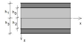
Fig. 1. Sandwich panel as a laminate structure
