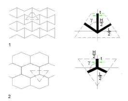
Fig. 2. Auxetic and honeycomb cellular structure with representative volume element
