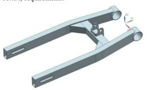
Fig. 3. Simplified 3D CAD model of suspension arm
