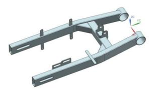
Fig. 2. 3D CAD model of suspension arm
