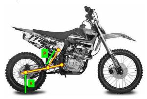
Fig. 4. Loading vectors layout
