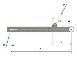
Fig. 5. Load vectors (P – load resulted from total mass of both vehicle and driver, R – ground reaction acting on the rear wheel, A – front bushes centre, b – distance between OX and OX1 axles, a – arm for projected force P)
