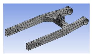
Fig. 8. Finite element mesh of suspension arm model (default system settings)
