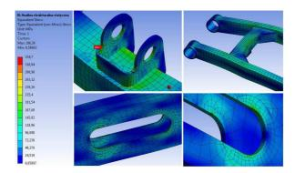
Fig. 10. The most loaded areas of suspension arm (MPa)
