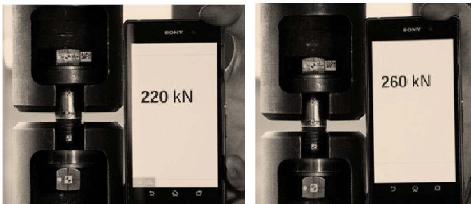
Fig. 8. Tensile test of bolt-washer-nut assembly (ISO 4014)
